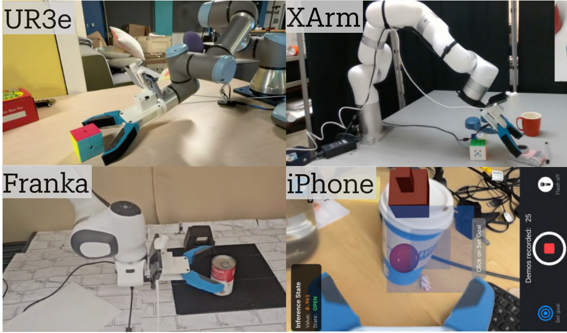
Figure 7: Cross-embodiment deployment of CAP on a Franka FR3, XArm 6, Universal Robotics UR3e, and an iPhone app. For the robots, the same CAP checkpoint generates EE-space motion that we translate to joint position control with IK. For the iPhone, the user is prompted to move the iPhone to where the robot should go next.
