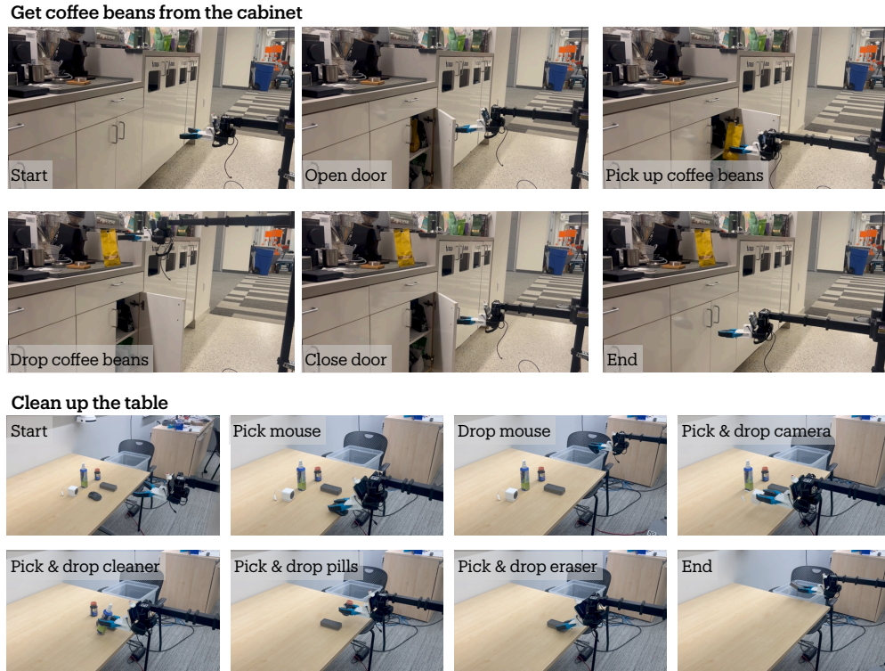
Figure 9: Performing long-horizon manipulations with Contact-Anchored Policies controlled by a high-level VLM controller via tool-calling. On the top, to retrieve coffee beans from cabinet, a controller combines Pick, Open, and Close CAPs, while on the bottom, a table cleanup is performed with Pick CAP.
